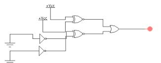
xiii.  $(A\overline{\bigoplus}B).(\overline{A}\ \overline{\bigoplus}\ \overline{B})$
